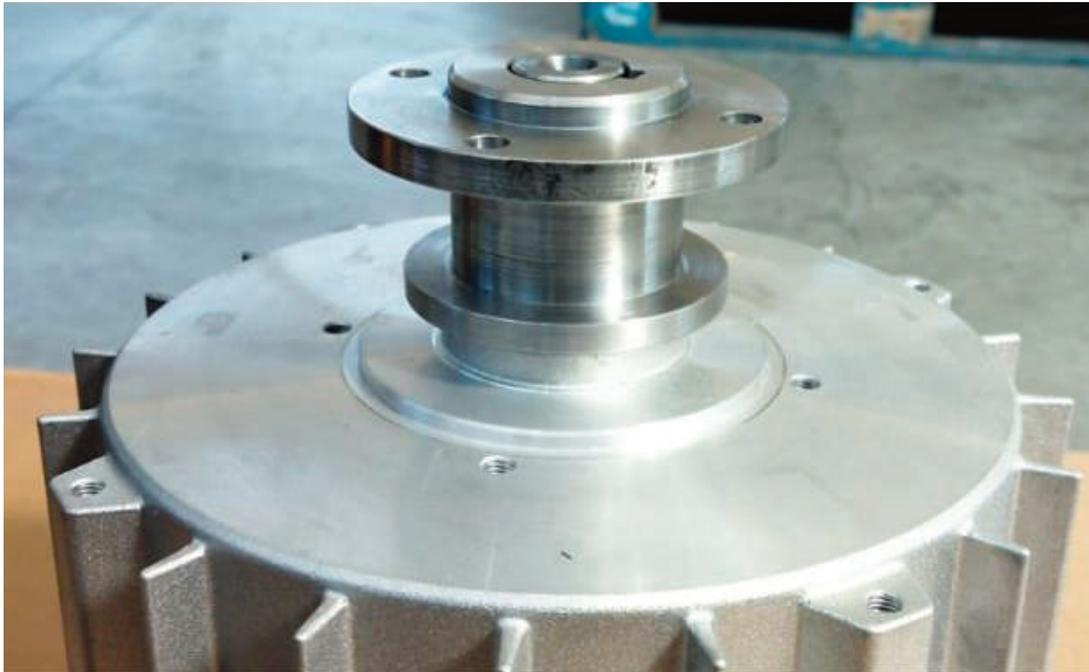
Slide off the fall protection plates and remove the hub from the shaft
