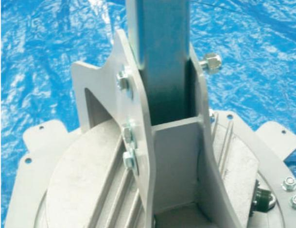
UNSCREW THE SCREWS FIXING THE ROD
